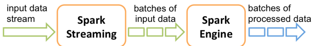
Figure 5.4 - D-Stream is a major concept in Spark Streaming
